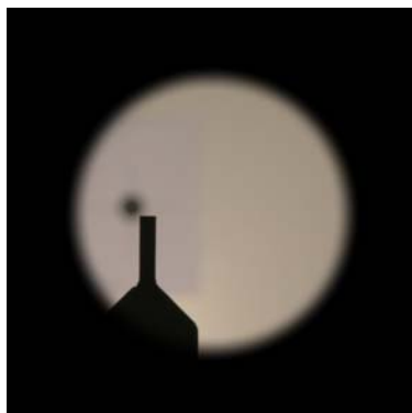
Rear sight out Eye shift left 1.25 mm
